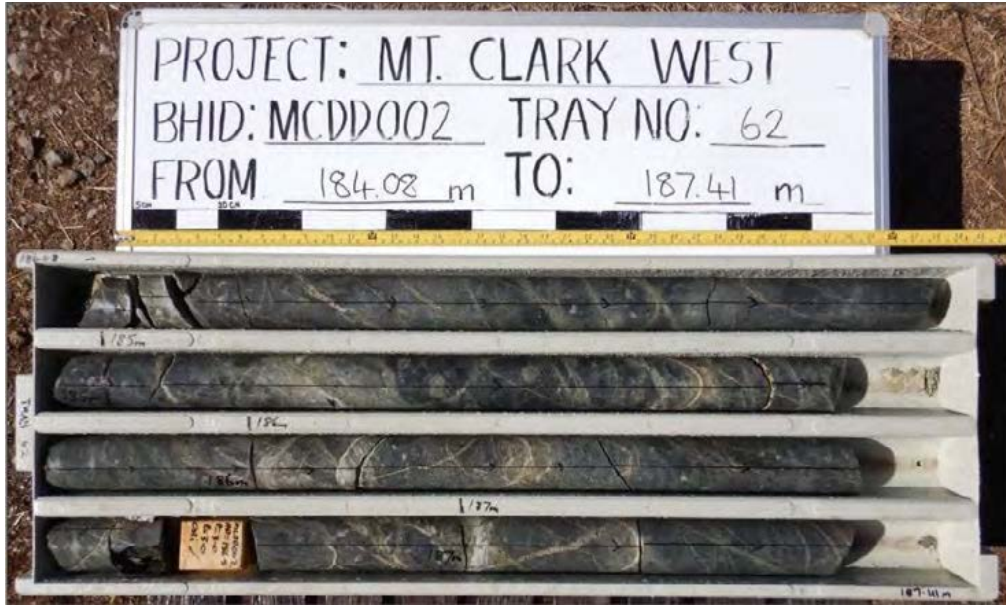
Figure 6-15: Drill Core Tray from MCDD002 Showing Part of the Interval 14 m at 0.23% Cu (Note the high level stockwork quartz veining and sericite alteration, indicating not yet in core of the system)
