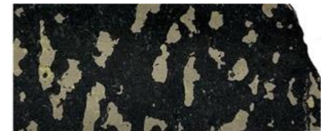
Globular sulfide from Oval Cu-Ni deposit in Mongolia. Photo moderate-to-coarse grained amphibole-olivine gabbro from DH OVD 008. XRF result is pending.
