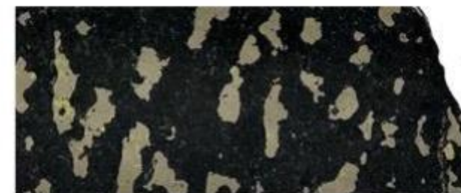
Globular sulfide from Oval Cu-Ni deposit in Mongolia. Photo moderate-to-coarse grained amphibole-olivine gabbro from DH OVD 008. XRF result is pending.
